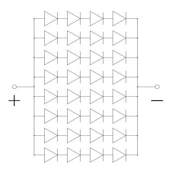
The voltage of each chip is range from 3.0v to 3.2v and e ach branch with maxium 350 mA current, so we can make t he design according the custo mer's requirement.
